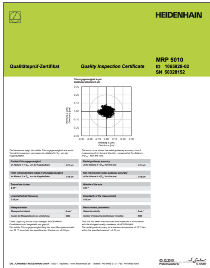
The Quality Inspection Certificate documents the radial guideway accuracy.
